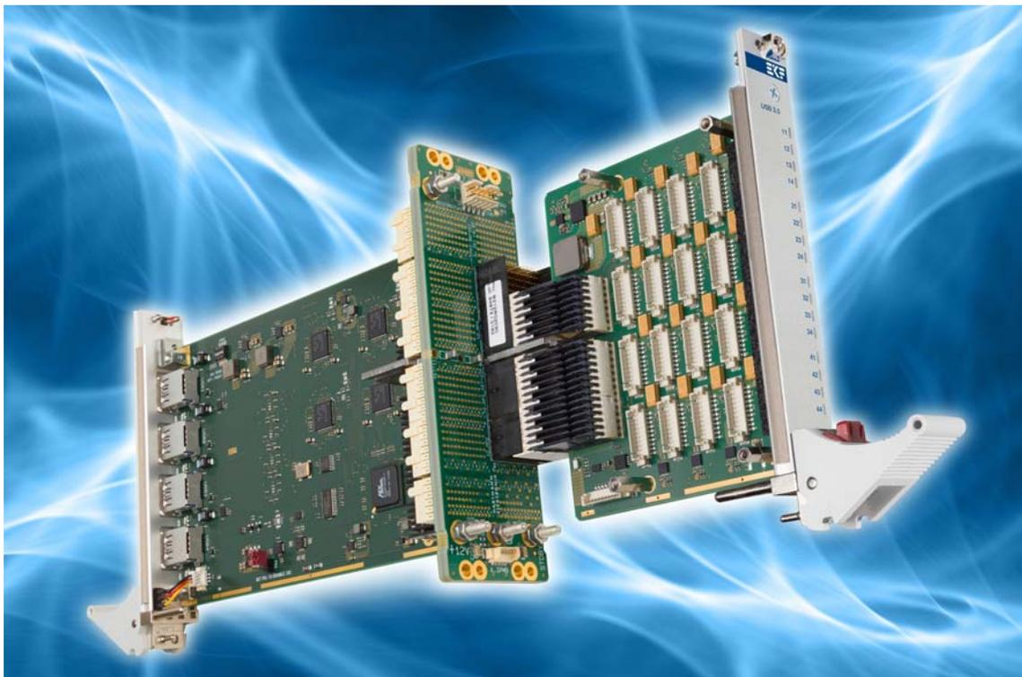
Board Assembly w. SBV-0200-RIO for System Internal Cabling
