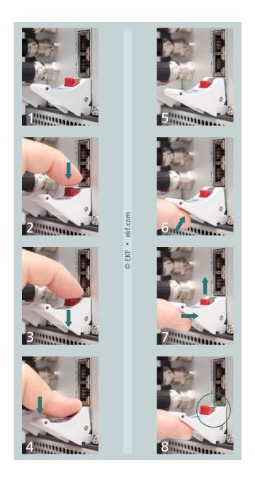
1 - 4: remove board 5 - 8: install board
