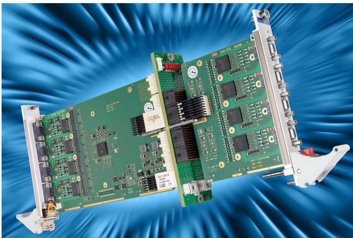
SUA-RIO w. SU1-TWIST (Isolated RS-485 Front Ports)
