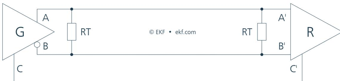
G = Generator • R = Receiver • RT = Termination Resistor
