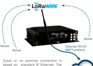
Cloud or on premise connection is based on standard IP Ethernet. The gateway automatically transforms LoRaWAN™ messages to a secure MQTT stream that is "pushed" on a remote MQTT server.
